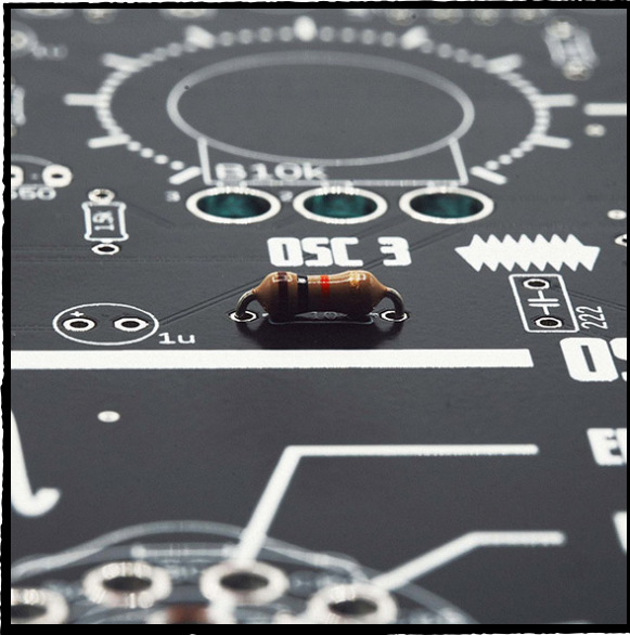
Image of resistor placed correctly.
