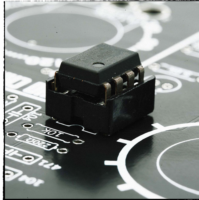
Image of ic placed correctly.
